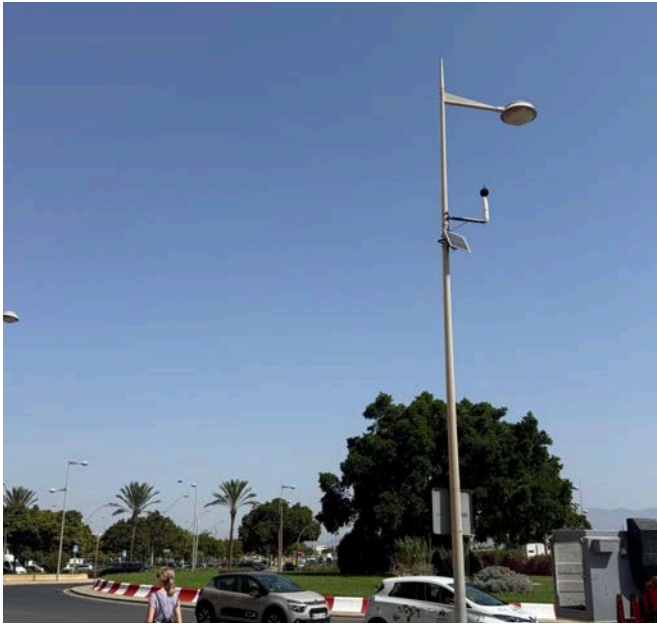
SVANTEK noise monitoring stations installed on street-lighting poles around the fairground, facing the nearest residential façades. Each station is self-powered by a compact solar panel.
