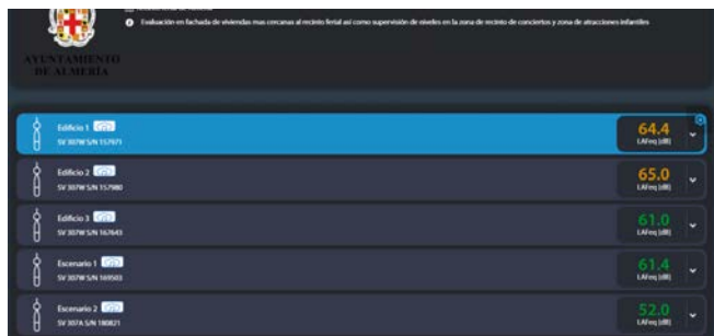
Live LAeq overview of the five SVANTEK stations (three façades, two stages) on the project dashboard.
