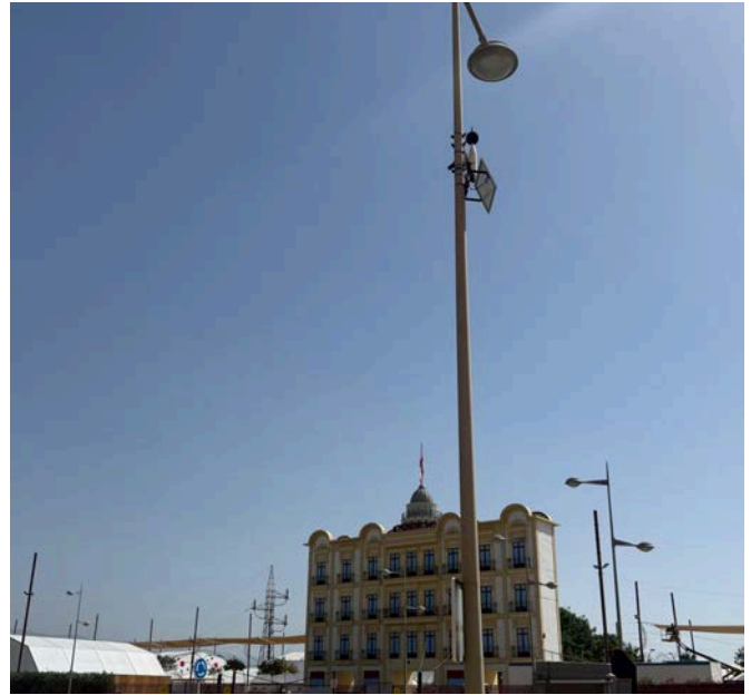
SVANTEK noise monitoring stations installed on street-lighting poles around the fairground, facing the nearest residential façades. Each station is self-powered by a compact solar panel.
