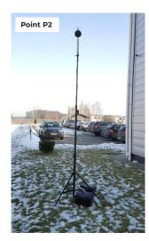
This setup allowed direct observation of the building's shielding effect on noise levels as a function of distance from the source.
