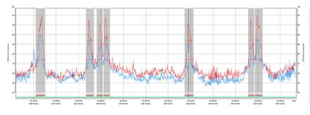
Detailed view of acoustic events (car passages) at observation points P1 and P2 with determined acoustic levels LAeqN for the nighttime period (8 hours).
