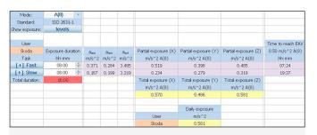
Vibration exposure values calculated in Supervisor software
