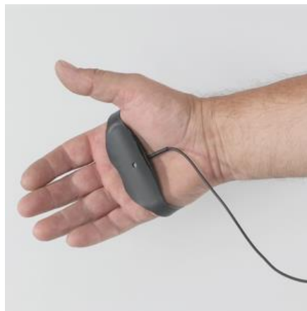
Photo 1 Hand-arm vibration adapter with tri-axial MEMS accelerometer and contact force sensor installed
