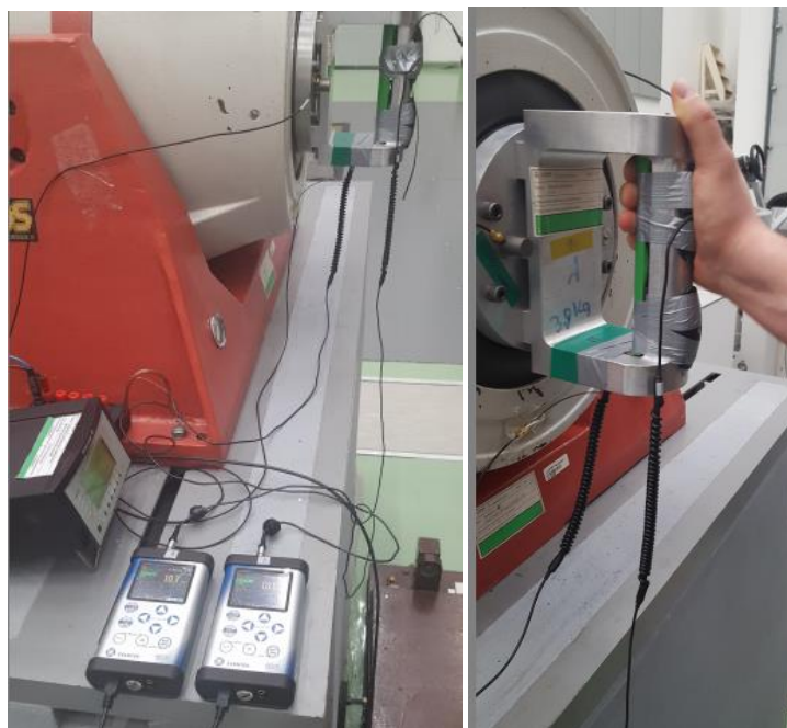
Photo 2 SV 106 meters with sensors and the reference accelerometer installed on the vibration exciter handle.
