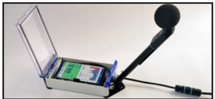
SV 302 – small stationary noise monitor with box for placing smartphone
