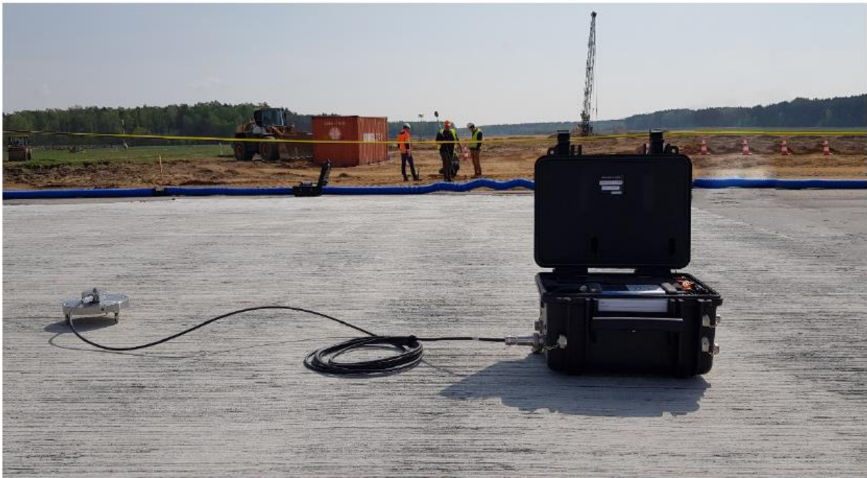
Picture 2 SV 258 PRO vibration and noise monitoring station.
