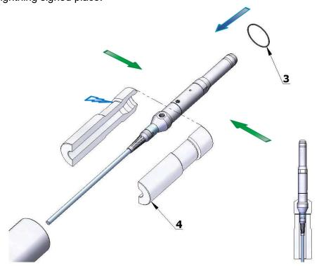
IV. Apply the upper, conical part (5) on the preamplifier.
