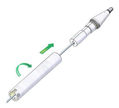
VI. Replace the dummy microphone (2) with the ½" microphone cartridge (B).
