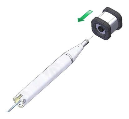
VIII. Install the microphone protection tube (6). Use the Allen key (K) as a pin at protecting tube orifice.
