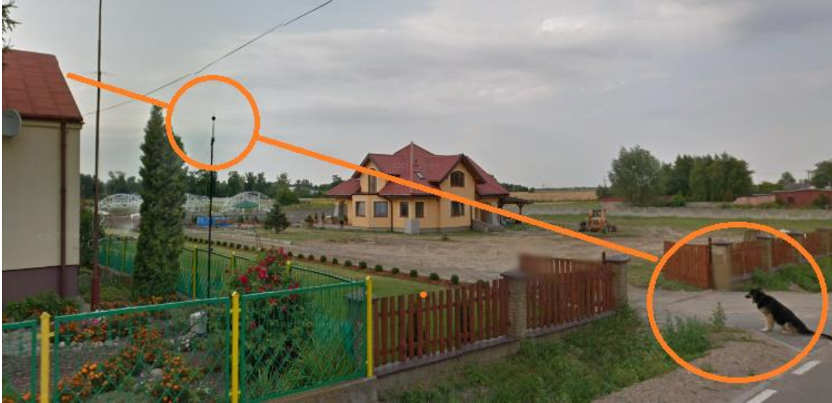
Picture 4 SvanPC++ Google Maps Street View mode indicating the SV 200A station, the dog and reflecting surface – the roof of the house.
