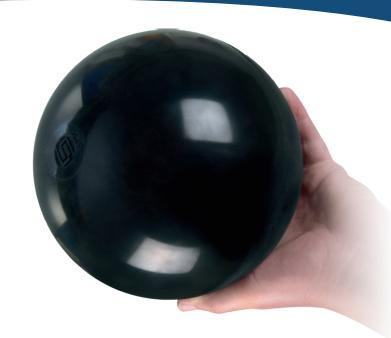
SP 95 Impact Ball is used for sound insulation testing in light weight structures where a standard (tapping machine) impact sound source would create too much impact force. It has been designed in accordance to ISO 10140-5 and ISO 16283-2 standards.
