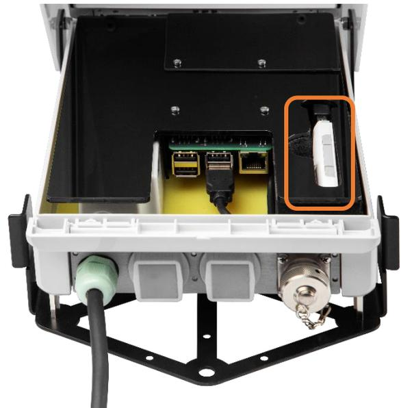
Then slide the cover to reveal the place for the card. After inserting the SIM card, you need to put the cover back and slide it towards the USB connector.
