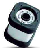
SV 34B Class 2 acoustic calibrator 114 dB at 1 kHz
