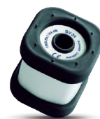
SV 34 Class 2 Acoustic Calibrator 114 dB at 1 kHz
