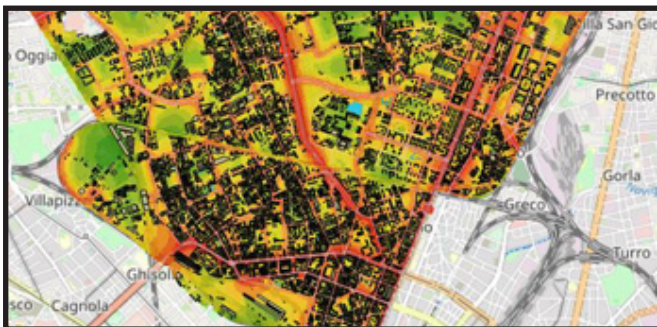
Example of dynamic noise map in city of Milan, Italy. Noise Exposure is updated every 30 seconds
